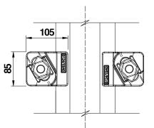
Minmum assembly width (W)=Rail Width(F)+170mm
