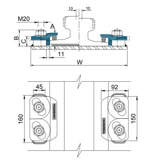
Minmum assembly width (W)=Rail Width(F)+130mm
