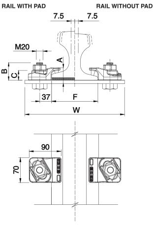
Minmum assembly width W=Rail Width(F)+147mm
