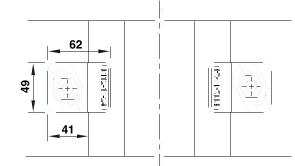
Minmum assembly width (W)=Rail Width(F)+92mm
